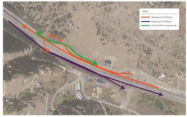
The Close Interchange at US 6 (move to east) concept, pictured above, moves the interchange to the east. Traffic from US 6 will need to go back up the hill. This options does not seem friendly to trucks or community. Intersections at both ends will be modified. Impacts are at the north side because all traffic will need to come up north side.
