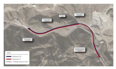
North Alignment concept – this concept held the profile high with a bridge. It comes up off the north wall or behind the valley (there is a significant profile shift in Floyd Hill).
